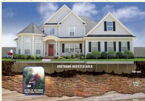
Chemical Grouting is used to stabilize shallow soils near the surface of your residence or pool deck. It is often used in the loose soil directly under your dwelling. In some circumstances, engineers may recommend a program of Chemical Grout Injection to stabilize the upper soils around the perimeter of the residence following a Compaction Grout Program and/or Foundation Underpinning Program.
