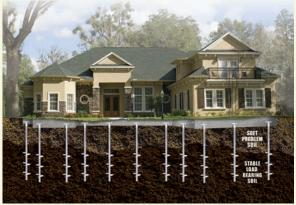
Helical Piers are the ideal solution for projects that are built on weak or wet soils and are prone to settlement. Piers can be installed in as little as 10' or as much as over 100'. Helical Piers are embedded into the concrete foundation during footer concrete pouring. Piers may also be attached to existing footers with the use of a wall plate.
