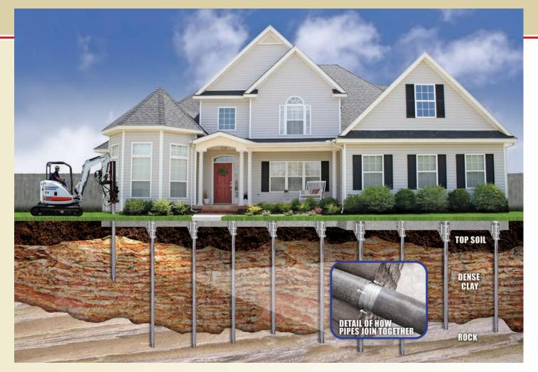
Underpinning is a method of repairing structures that have been damaged or have settled from sinkhole activity, buried organics, shrink/swell clay, etc. Underpinning supports the foundation of a structure by transferring the weight of the structure from the foundation through the unstable soils, to a more stable material below, which is typically limerock.
