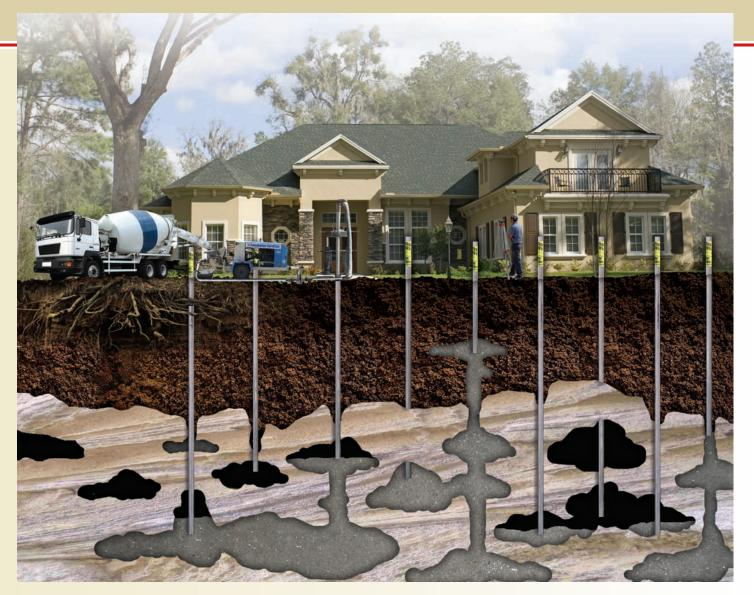
Sinkholes can cause tremendous damage to structures. Foundation Services performs pressure grouting in areas that geotechnical engineers have found to be sinkhole conditions. This involves the injection of a low slump grout into the soils at or above the limestone layer to seal the collapsed or eroded limestone, fill voids and compact loose soils.
