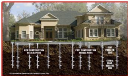
Installed piers are secure and undetected once the footer is covered.
